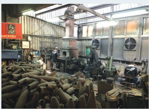
The Maestro Wu factory with its copious supply of steel shells. The WORKER ON THE LEFT IS MELTING A SHELL SECTION IN THE FURNACE, THE STAMP-ING PRESS IS IN THE CENTRE, WHILE ANOTHER WORKER POLISHES A BLADE.
